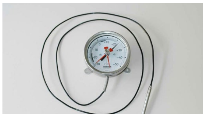
Figure 6. Fixed gas/vapour pressure-dial thermometer
