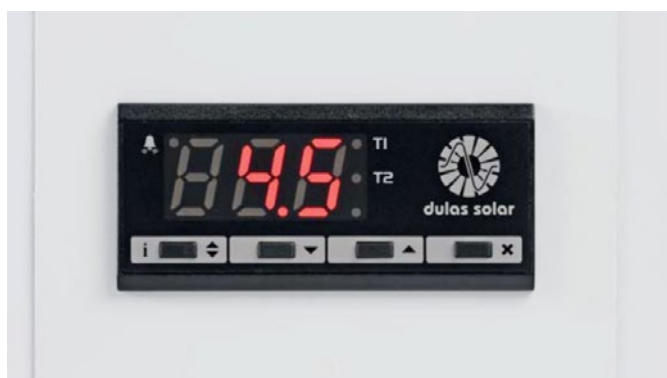
Figure 9. Integrated digital thermometer
