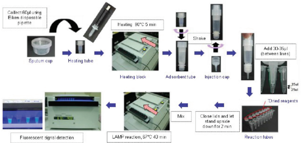
Figure 3. Schematic description of the workflow for TB-LAMP
